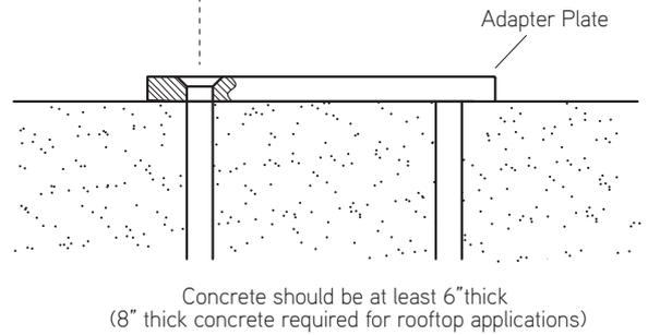
**3** Insert (4) expansion bolts into countersunk holes and tighten using an allen wrench.
