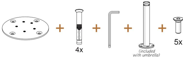
**1** Aligned countersunk hole and internal stem hole must face direction of umbrella! Drill (4) holes on concrete according to countersunk holes in diagram below. Hole depth should be no less than 4" / 100mm.
