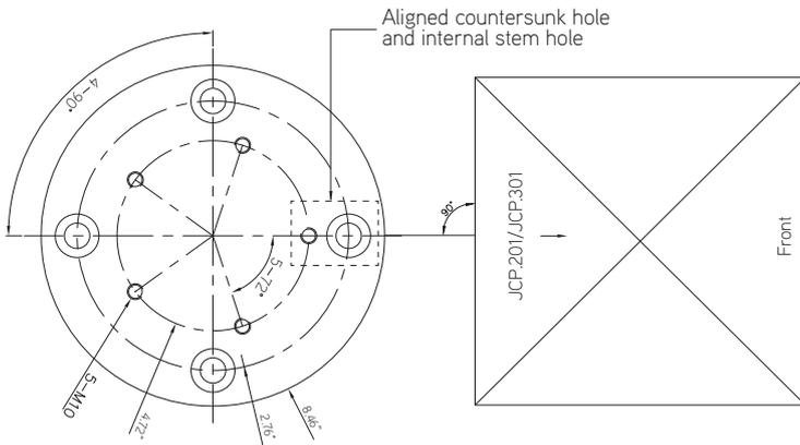
**2** Make sure all adapter plate holes align with drilled holes in concrete.
