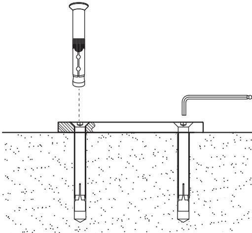
**4** Align internal stem holes with adapter plate holes. Insert (5) stem bolts and tighten using an allen wrench to secure. Note: Internal stem and stem bolts are included with the umbrella.
