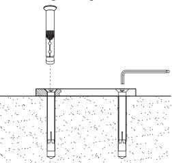
Align internal stem holes with adapter plate holes. Insert (5) stem bolts and tighten using an allen wrench to secure. Note: Internal stem and stem bolts are included with the umbrella.
