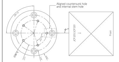
Make sure all adapter plate holes align with drilled holes in concrete.
