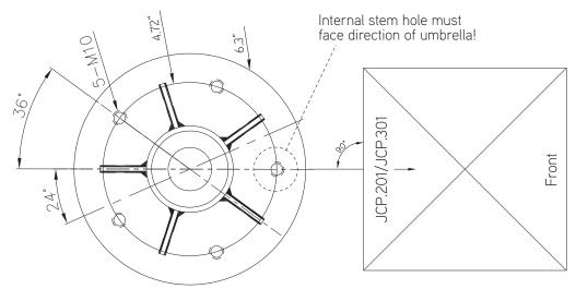
Dig an approximate 60cm/2ft. deep by 90cm/3ft. wide hole. Insert in-ground fitting and pour mixed concrete into hole around fitting. Make sure in-ground plate is level.
